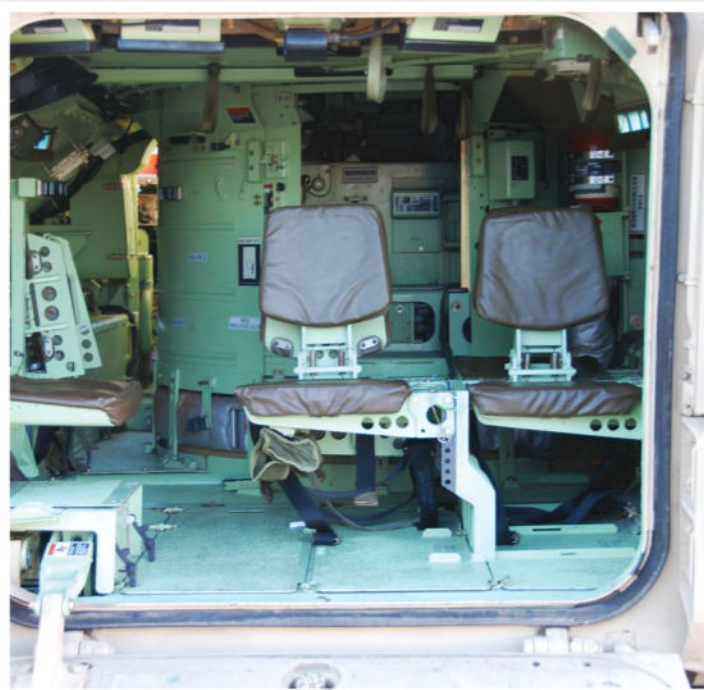
Above: The interior of the M2/M3 Bradley Fighting Vehicle is compact but functional in either infantry or cavalry configuration
