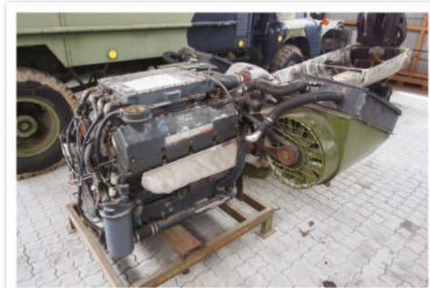
Above: The Cummins VTA903T diesel engine powers both the M2 and M3 Bradley Fighting Vehicle variants
