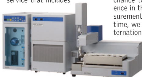
AQF-2100H for combustion IC for PFAS screening
