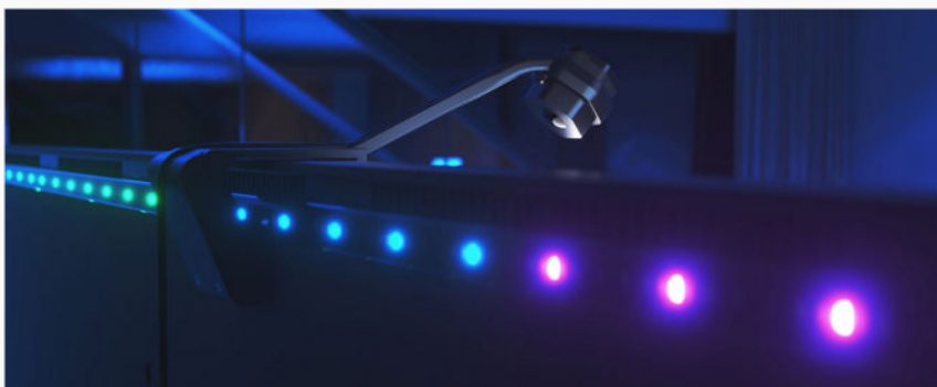
The camera keeps an eye on your TV screen so it can match the colours to the light strip.
