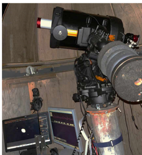
▲ Jane's observatory setup with ZWO ASI662MC (right), Celestron scope and driven mount all linked to her PC
