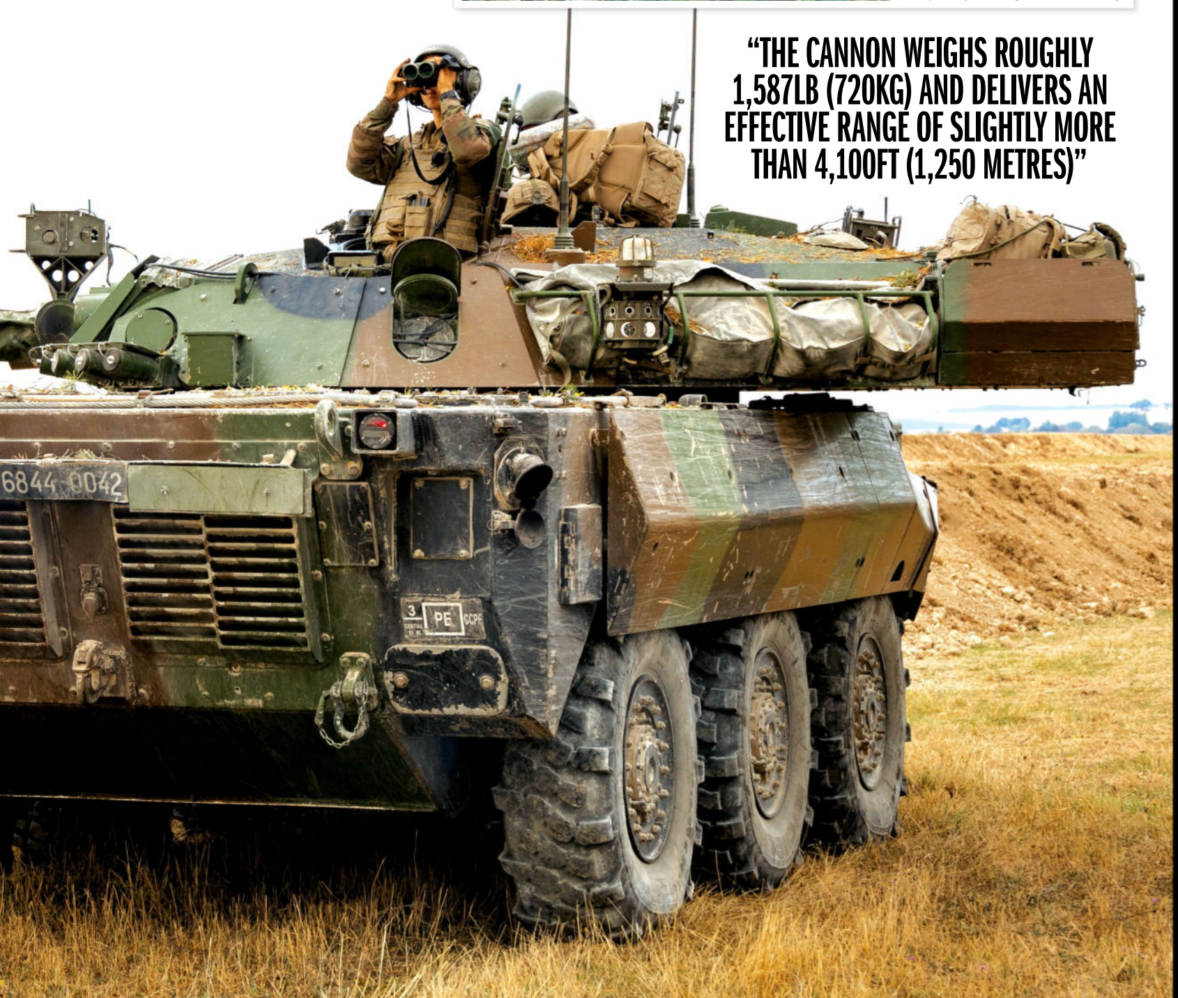
The AMX-10 RC was originally designed as an amphibious vehicle, but that capability was negated with refitting
