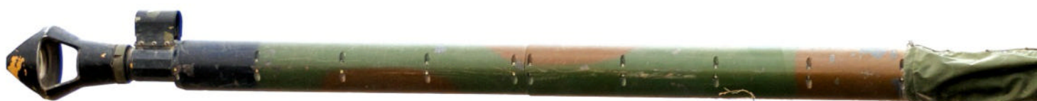
The barrel of the 4.1in (105mm) F2 BK MECA L/47 cannon features shallow rifling and high muzzle velocity
