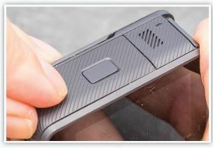
Once battery and memory card are in place, you can close the compartment lid so it slides and locks into place. Your camera is ready to switch on.
