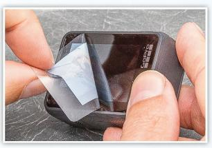
Now you can simply slide the camera out of its frame. There is a plastic screen cover on the LCD, you can peel this off.
