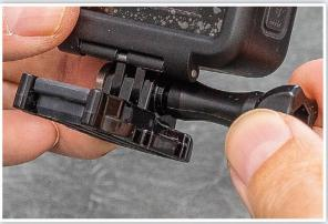
You can then put the thumbscrew back in and tighten it up. The thumbscrew holds the GoPro frame to the mount.
