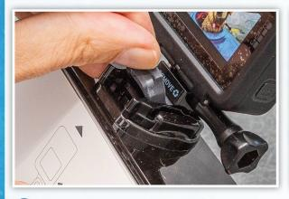
Let's take a look at the camera itself. The camera can be removed from the display box mount by lifting the rubber stop.
