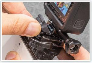
You can then squeeze the two mounting clips together and then slide the GoPro off the mount.
