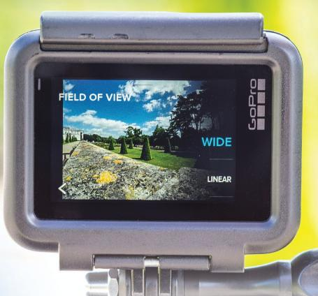
OV refers to how much of the scene you are shooting can be seen by the camera via the lens. FOV is measured in degrees. The greater the angle in degrees, the wider the view and hence more of the scene is captured. You FOV options are based upon what resolution and frames per second video settings you are using.
