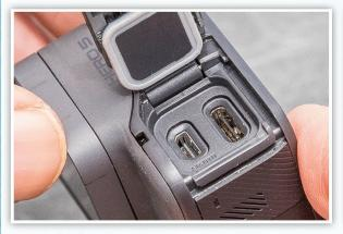
Now you can have a look at the two camera compartments. The first, on the side by the lens, contains the HDMI and USB-C slots.
