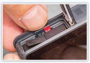
You can use your fingernail to make sure it is firmly seated by pressing it down into the slot until it locks into place.
