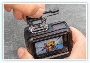
To remove the camera from the frame, you need to release the securing clip on the top. This lets you swing the back of the frame down to remove the camera.
