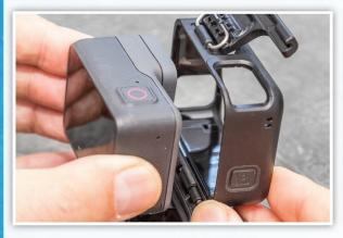
You can put the camera back in its protective frame and snap the securing clip shut.
