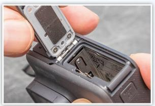
Underneath the camera is the battery compartment and the slot to house the Micro SD memory card.
